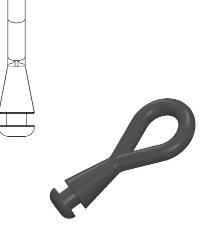
Recommended hole dimension is 0.125" with center at the line where the two parts come together.
